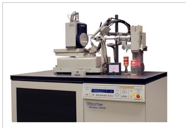
Figure 1: Microfocus source in-house diffraction system comprising 007 rotating anode generator, Confocal Max-Flux variable dispersive optic, CCD detector mounted on quarter chi goniometer with cryo-cooling device.
