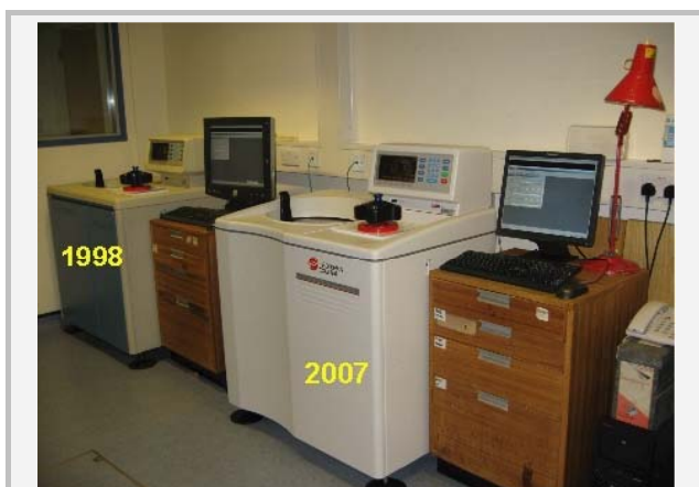
Figure 1. Equipment. The AUC laboratory is pictured with both instruments side by side. For these, we possess four-hole and eight-hole rotors and sets of six-sector equilibrium cells and two-sector velocity cells. AUC data are saved onto a networked server and permanently archived. Data processing is performed in a computing laboratory supported by the latest DCDT+, SEDFIT and SEDPHAT software packages in which we are expert, helped by our home-written "easy-to-read" manuals. If required, sample and buffer densities can be measured on an Anton-Paar DMA 5000 densitometer.
